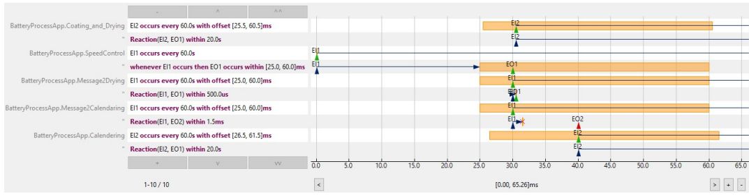
(a) Failed execution time trace, because the message transmission of M_SC took too long.
